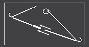
b. Push the angled arms of the gambrel down and together simultaneously until they flex close enough together to push the ring over the hook on the opposite side.
